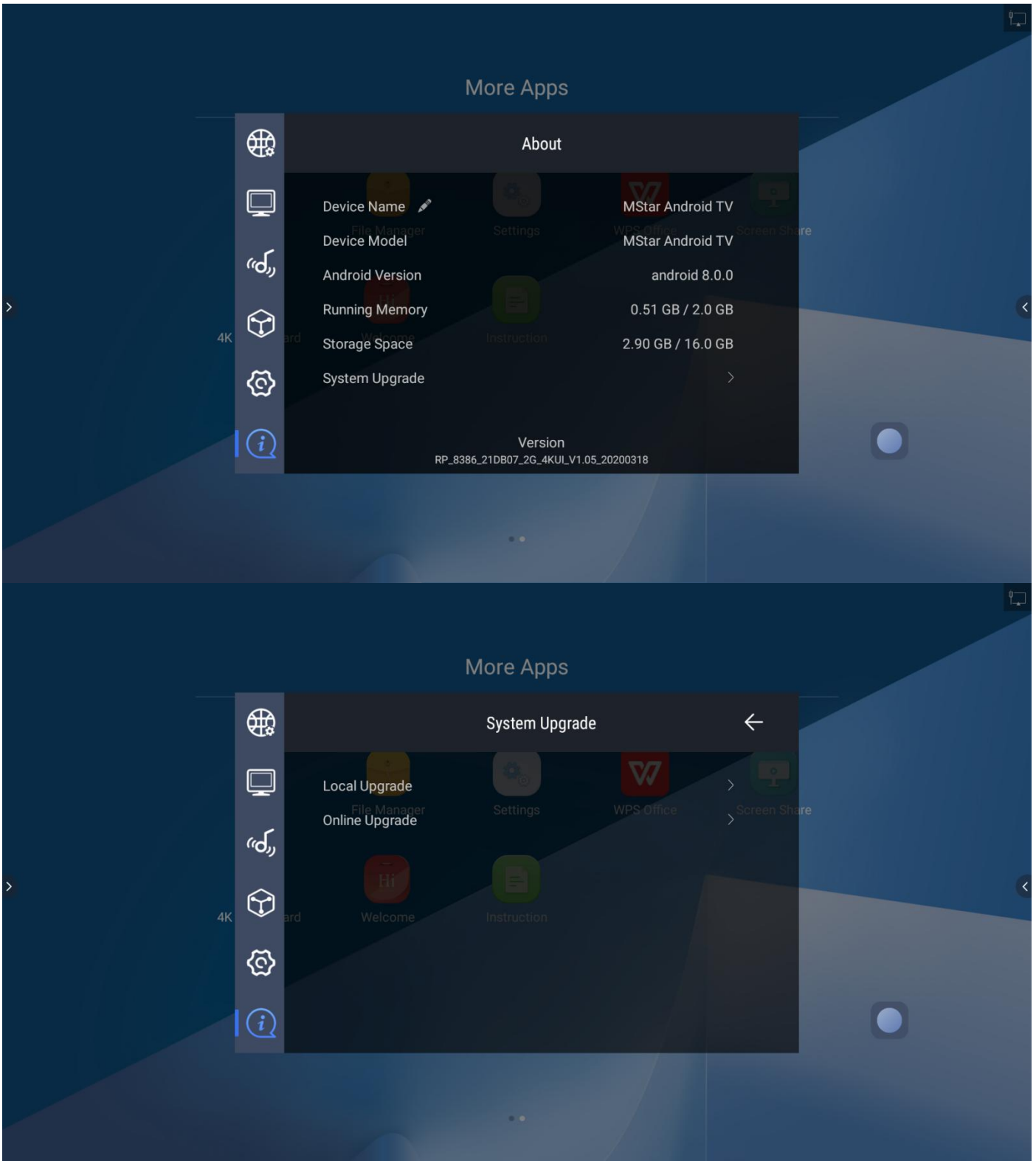
4.6.1 Device name Click the device name to rename the device.
